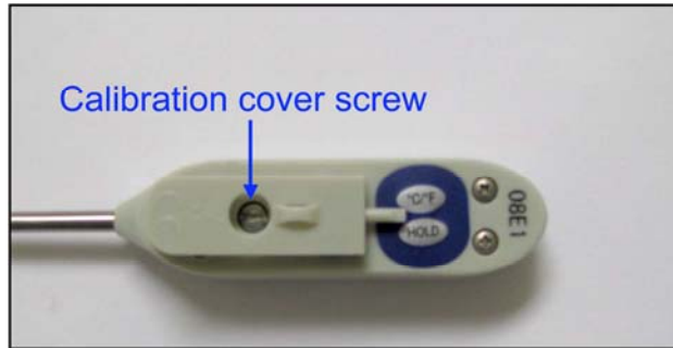
Figure 1: Cover screw to access calibration potentiometer
